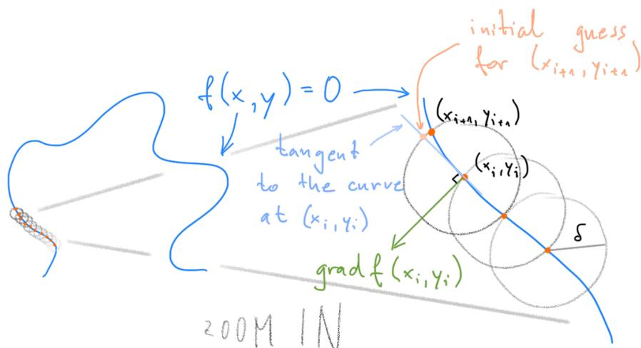
We are trying to construct **orange** dots. Suppose we are currently at the point  $(x_i, y_i)$ . To construct the next **orange** dot, we'll move along the **tangent** through the point  $(x_i, y_i)$  for a step of length  $\delta$ . This will give us an **initial guess**, and Newton's iteration will (hopefully) converge to the next **orange** dot - the point  $(x_{i+1}, y_{i+1})$ .
