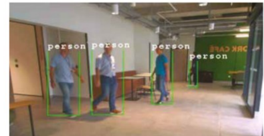
People detection and tracking Yolo v8 320x320 Neural-ART with 4 Convolution Array at 1 GHz = 26 fps
