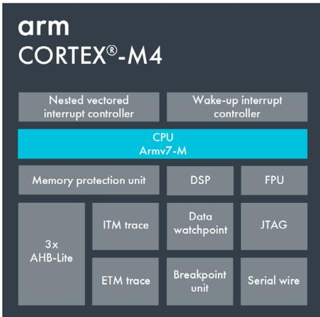
Figure 1: Block diagram of the Cortex-M4 processor
