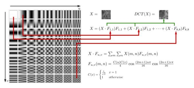
First component is direct current (DC) offset and represents the mean value in the block. Remaining components are alternating - AC
