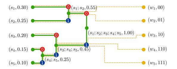
Naive encoding (3bit codes) – 15 bit  $s_1, s_3, s_1, s_2, s_2 \rightarrow 010001010011011$ Huffman encoding – 10 bit  $w_1, w_3, w_1, w_2, w_2 \rightarrow 0010000101$
