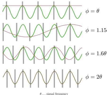
$\theta \dots$  signal frequency  $\phi \dots$  sampling frequency
