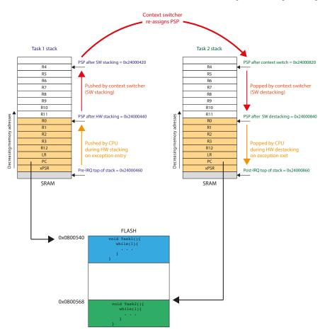
Fig. 1.20: The modification progress of the PSP stack pointer during context switching.
