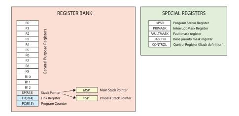
Fig. 1.10: ARM Cortex-M7 core registers.
