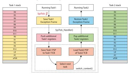
Fig. 1.19: Context switching using stack pointer swapping.
