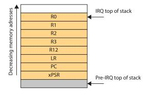
Fig. 1.14: The layout of the stack frame after stacking in ARM Cortex-M7.
