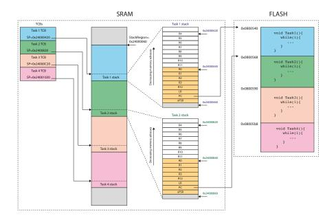
Fig. 1.18: Memory layout and content after creating four tasks.
