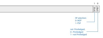
Fig. 1.12: CONTROL register.
