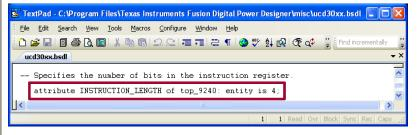
Modify, or create the file "idcodes.lst" to include the device ID (reported by JTAG loader) and the IR Register \_ Length (from the BSDL file).
