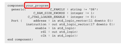
Paste the program memory component declaration into the appropriate section of your design file (i.e. after 'architecture' and before 'begin' in VHDL).
