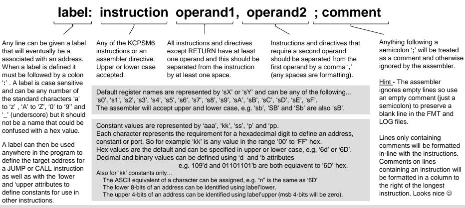
Assembler directives follow the same basic syntax but are only used to direct the assembler and make code easier to write and understand.
