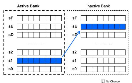
Example STAR SE, S1 'SE' in the inactive bank is loaded with a copy of 's1' in the active bank (illustrated in the diagram above).
