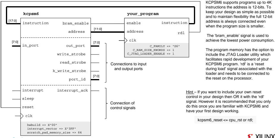
when the program size is smaller. The 'bram enable' signal is used to achieve the lowest power consumption.
