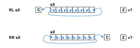
RL sX shifts all bits one place to the left and the MSB that is shifted out is shifted into the LSB as well as copied into the carry flag. The Z flag will only be set if all bits of the register are zero.
