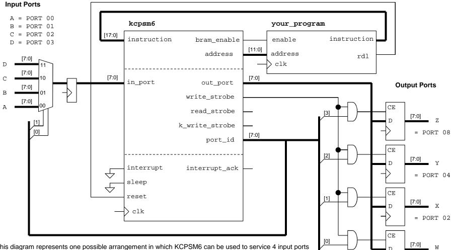
This diagram represents one possible arrangement in which KCPSM6 can be used to service 4 input ports and 4 general purpose output ports. Each port is up to 8-bits and could be connected directly to pins on the device package or may connect to some of your other logic within the device. All KCPSM6 designs build on variations of this fundamental arrangement. Suitable PSM code for this circuit is shown on page 51.
