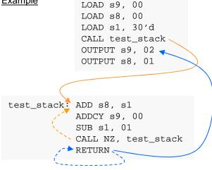
This example illustrates the general arrangement in which one part of the program calls a subroutine. In most cases line labels are used to make the code easier to write and maintain and the assembler resolves the actual addresses.
