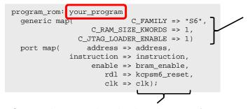
Connect the appropriate signals to the ports. If you used the default signal names then nothing needs to be modified.
