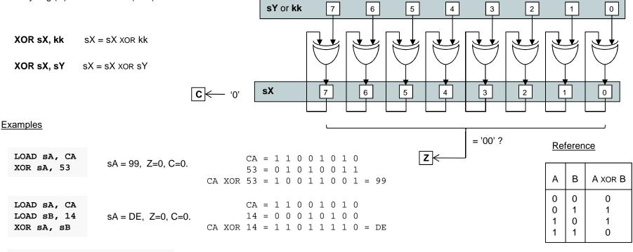
CONSTANT strobe, 00000001'bHint - The XOR instruction can be used to toggle the state of bits within a register. In this example the least<br/>significant bit of 's0' is twice toggled and output to a port. Assuming the LSB was '0' to begin with<br/>then this will have generated a positive ('1') pulse on the LSB of the output port whilst all other bits<br/>remained unaffected. The CONSTANT directive provides a convenient way to name bits that you<br/>may wish to control in this way.
