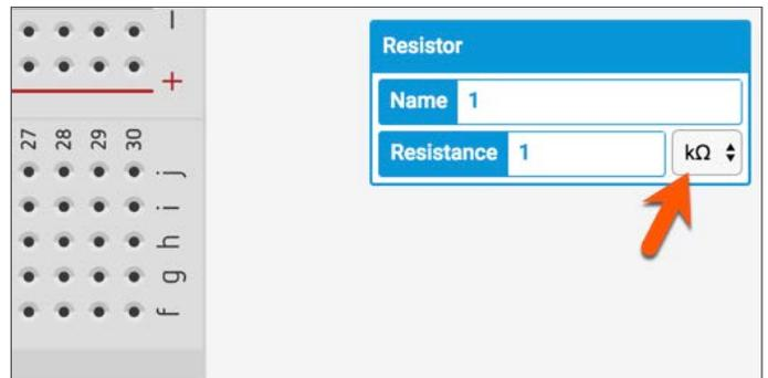
Click the symbol selector to see other measurement symbols for Ohms. There is a total of eight. We won't be using most of these measurement symbols. I want to point out a few that will be used in this and other chapters.
