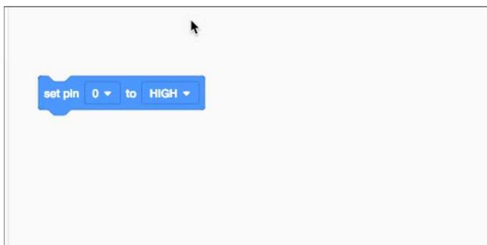
Change the pin argument to 3. The second argument has two states. A state has one of two options. A state can be on or off. In this code block, the state is set to high. A high state is the same as an ON state. The other option is a low state. This is the same as OFF. Computers read everything as either ON or OFF or ones and zeros. Binary numbers like one and zero are at the heart of all computers.
