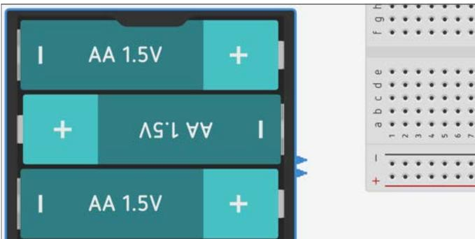
Connect jumper wires from the negative battery terminal to the negative rail on the breadboard and connect a jumper wire from the positive battery terminal to the positive rail on the breadboard.
