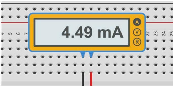
Click on the letter “V” on the meter to read the voltage. The voltage is 4.50. Dividing these two numbers will give us 1 kilo-ohm.
