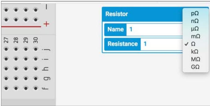
Make sure the resistance unit of measure is set to kilo-ohms and click the Start Simulation button.
